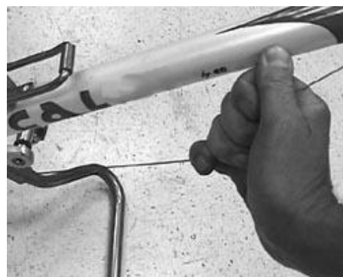
Test the shifting by pulling the inner wire
